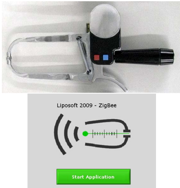
Figure 2. LipoTool integrating sensing and wireless communication system.
