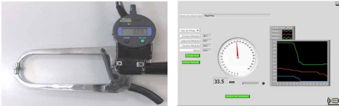
Figure 1. LipoTool with a Harpenden SC adapted with a digital dial indicator.
